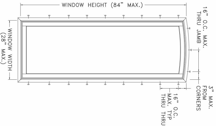
TYPICAL ELEVATION WITH FASTENER SPACING
